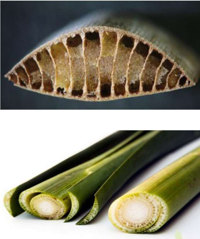
Photos 46-48. Left: leave (above) and stalk (below) of Typha and a construction board made from Typha (right)
