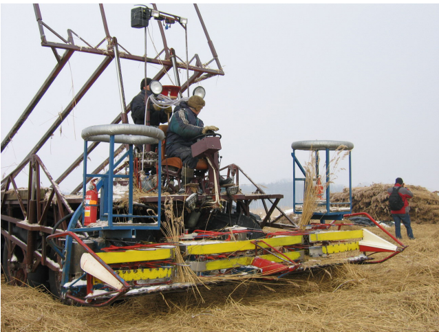
Photos 24 – 25. Reed mowing with a Seiga-like harvester and transport of reed bundles after manual combing and bundling in Rozwarowo, Poland (Wichtmann 2006)
