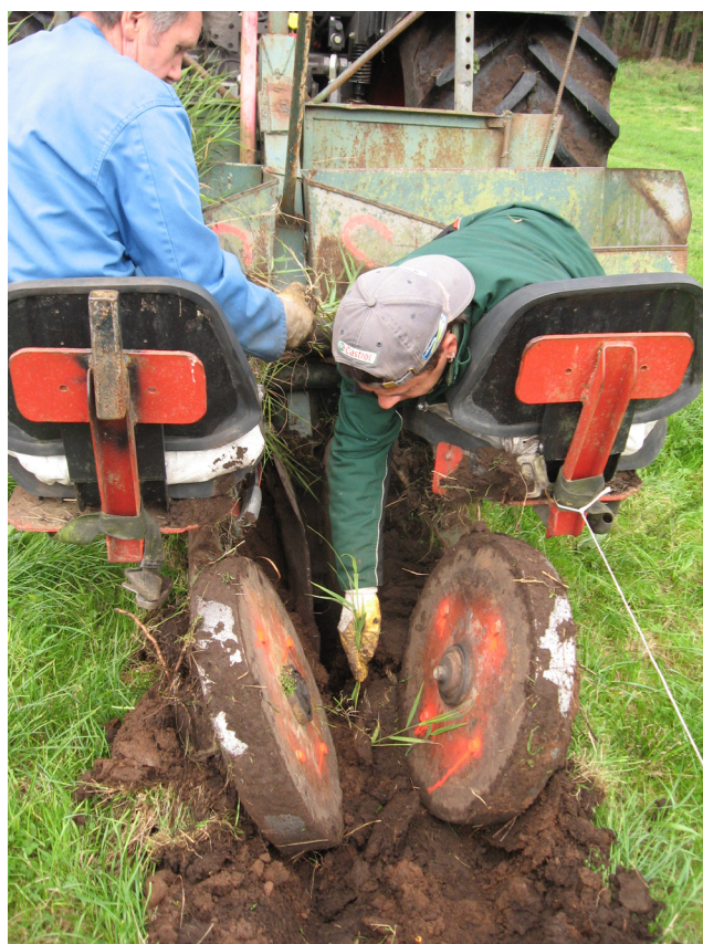
Photo 30. Planting using a forest planting machine (Wichtmann 2008)
