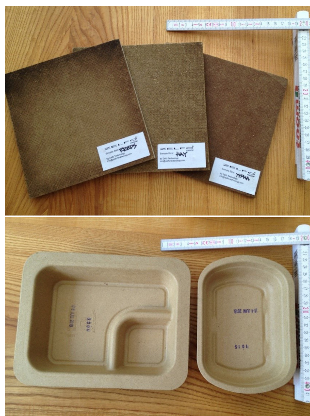
Photos 17 and 18: Construction plates (left) and compostable disposable tableware (right) pressed from unspecific biomass from wet meadows (Wichtmann)
