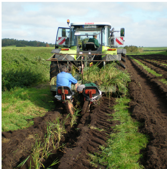
Photo 29. Planting using a forest planting machine (Wichtmann 2008)
